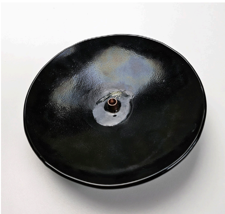
Image 7: Underside of cap with epoxied stemming hardware
