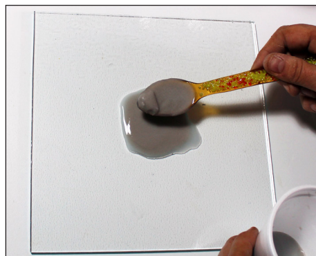
Create a slurry with Bronze (refer to Red Dashed Box above). Place the slurry into the center of the square, then shake the glass gently from side to side to evenly disperse it.
