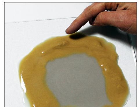
Create a slurry with Medium Amber and add it in a circle around the Bronze center. If you see areas where frit is clumping, gently shake the sheet glass to settle them.
