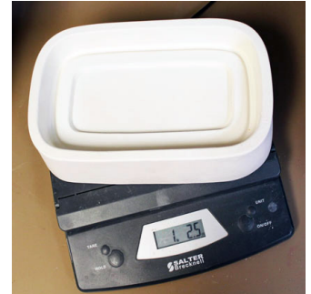
Image 10: Empty primed mold atop scale.
