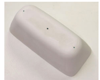
Image 6: Primed mold with pencil marks
