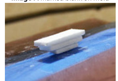
Image 8: Stacked Fiber Paper for draping handle
