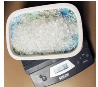
Image 11: Frit-filled mold atop scale.
